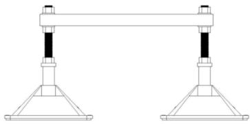
The StrutFoot Beam is an adjustable heavy duty support system which is typically used with heavy Air Handling Units (AHU's), chillers or when existing steel beams need to be picked up on the roof.
